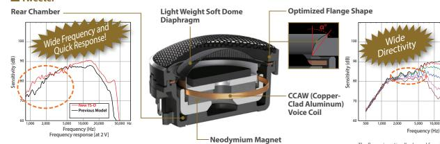
$The new D-Series components are capable of wider frequency sound and \ quicker response in playback than any models that preceded them.$
