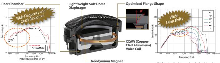
The new D-Series components are capable of wider frequency sound and quicker response in playback than any models that preceded them.
